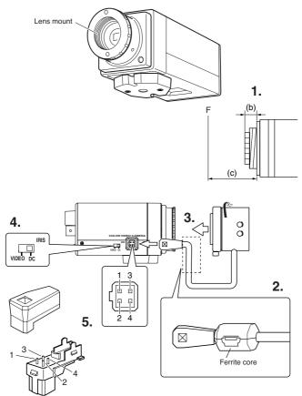
Before mounting a lens, check whether it is CS-mount lens. Dimension (b) of the lens shown in the illustration must be as shown in the table below. If (b) exceeds the value in the table, it may damage the inside of the camera or correct mounting may be impossible; never use such lenses. The F mark indicates a focal point.
